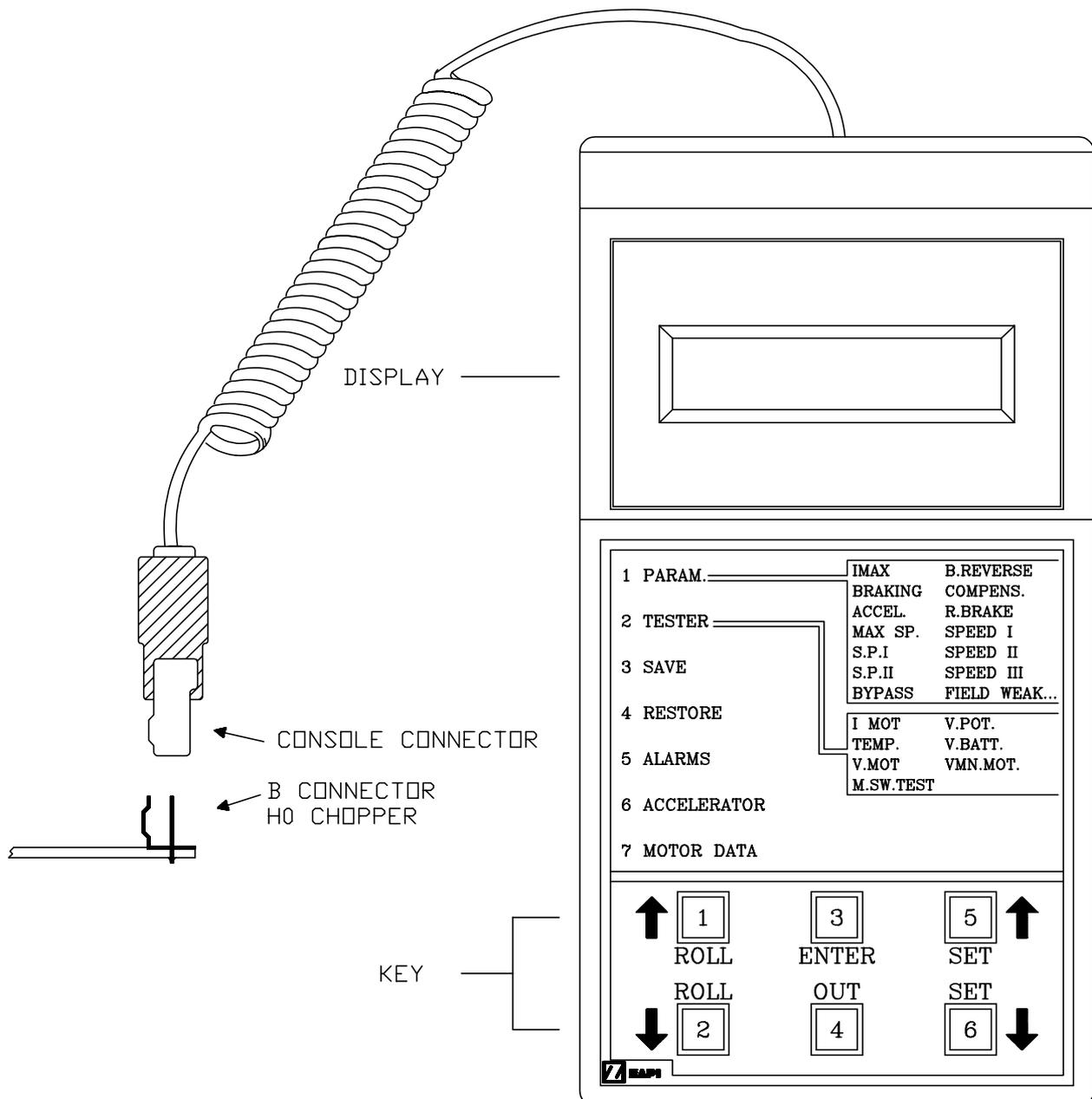
The console to be used for H0 chopper shall be equipped with CONSOLE eprom release 2.00 or following.
