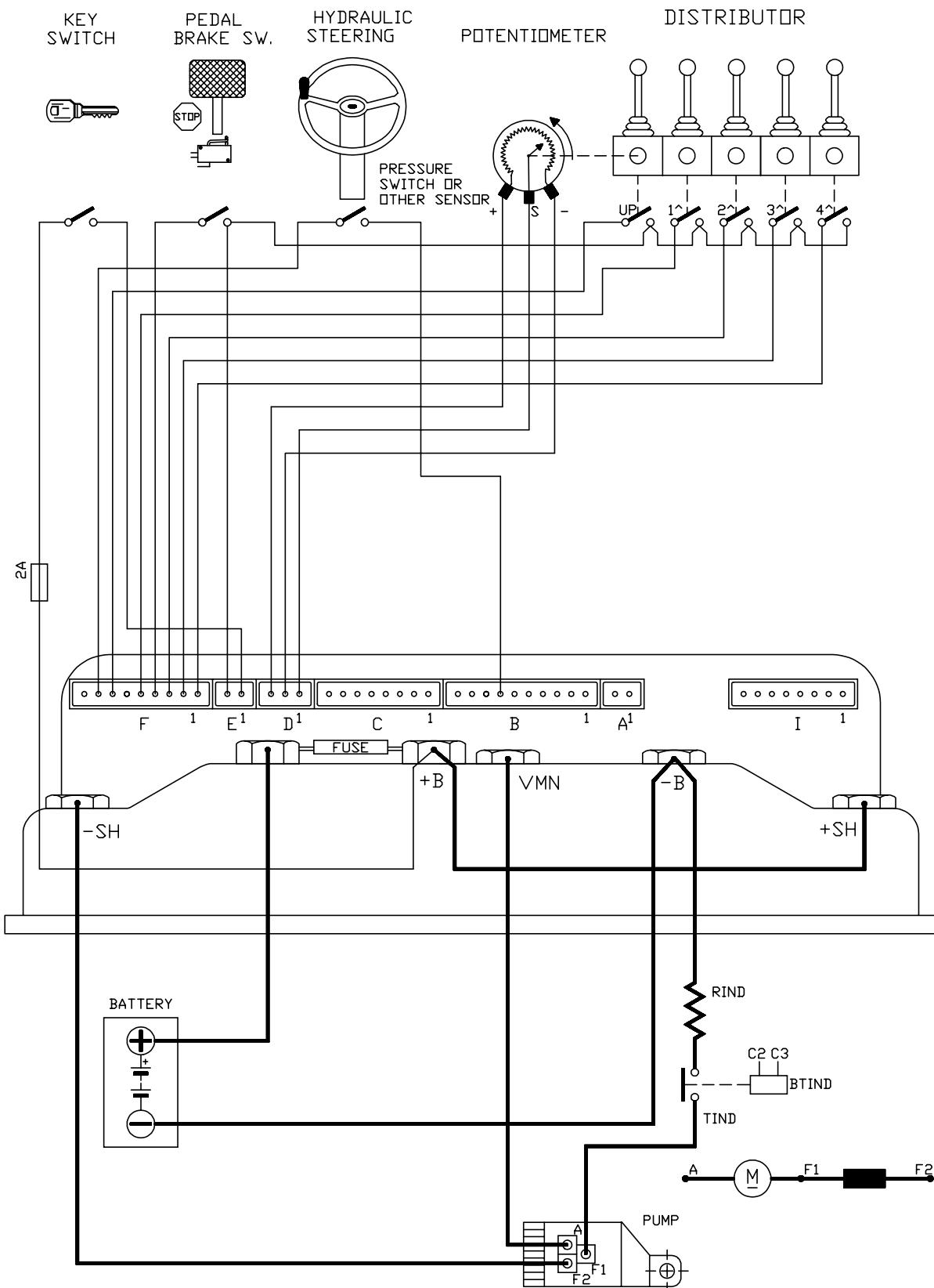
**8.7 WIRING DIAGRAM FOR H3D STANDARD LIFTING WITH BYPASS AND MAIN CONTACTORS. POWER STEERING COMMAND FROM RUNNING CONTACTORS (\*)**
