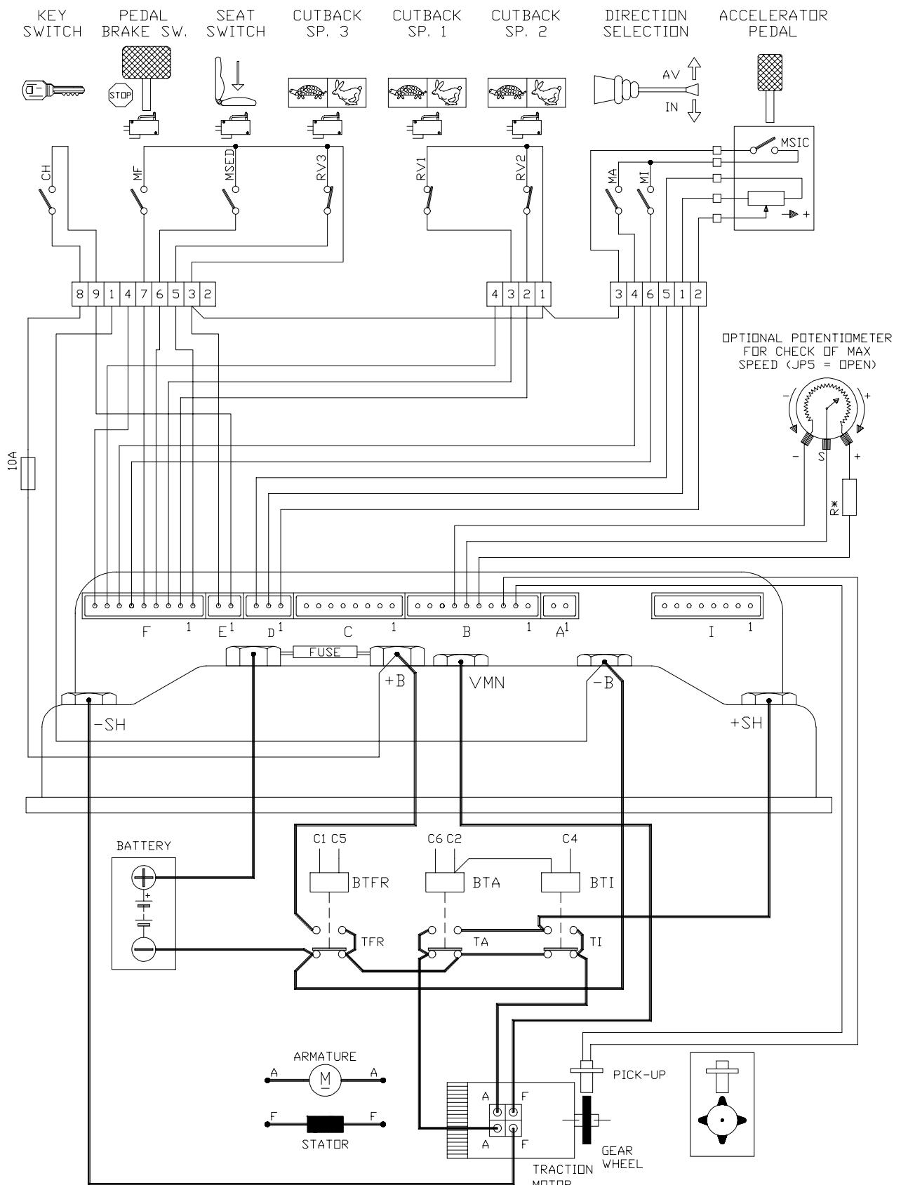
⚠ R\* = The value of the resistance is double than the one installed in the potentiometer; it is necessary for limiting the regulation range.
