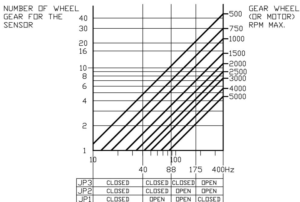
Example: The requests are revolutions 2500 RPM max and on the drive shaft is connected with a 4 - gear wheel. For the selection of the jumpers positions point from the scheme where the 2500 rpm line crosses the 4 - gear line, then modify the jumpers like as in the table under the scheme; in our case it has to be used the table from 88 kHz to 175 kHz.
