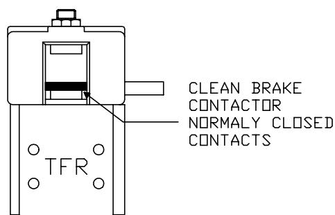
It could be necessary to replace the contactor.
