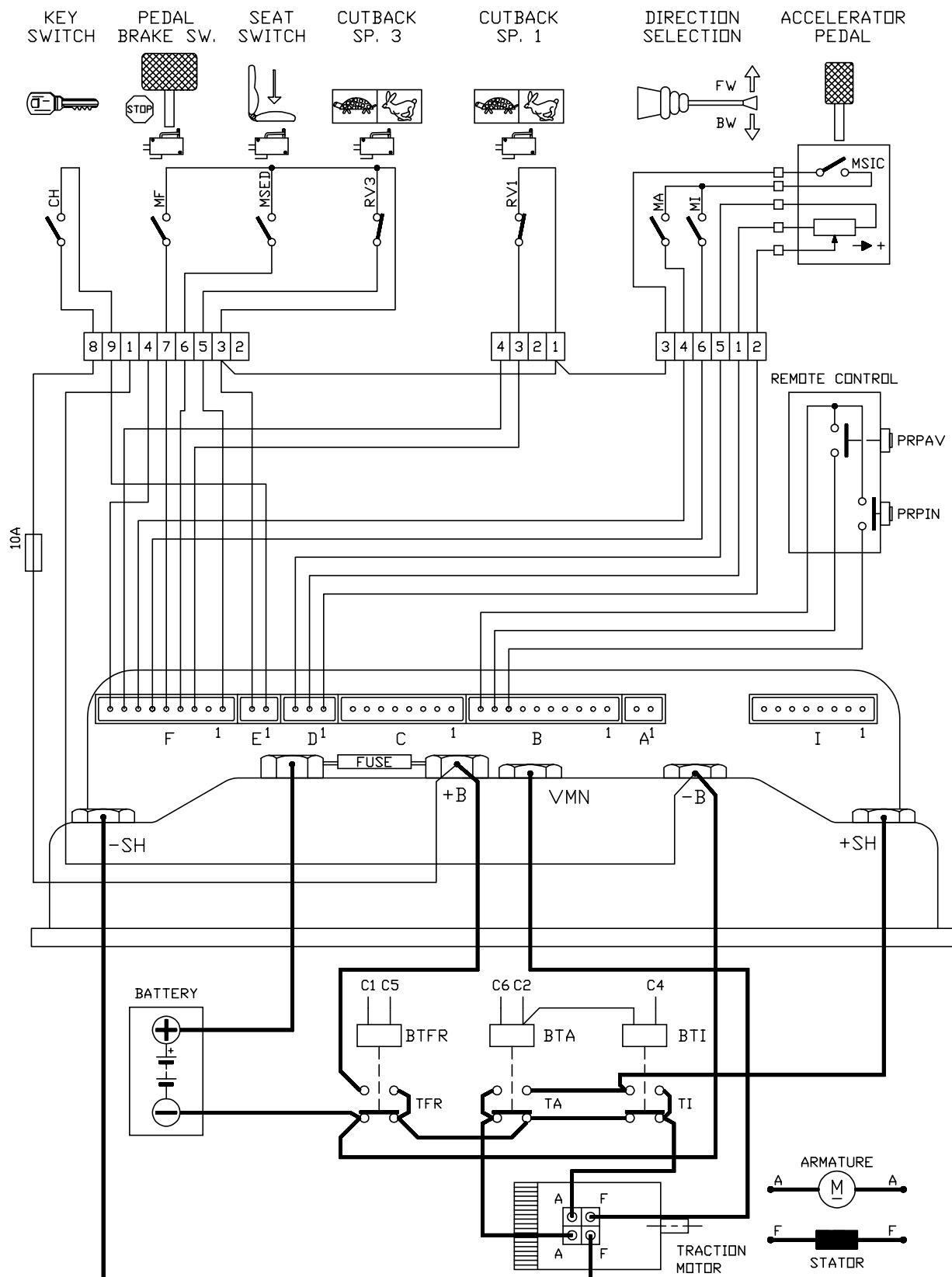
⚠ N.B.: For the operating of the backing request, program the option PIN F2 in the BACKING mode.
