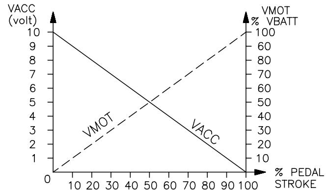
VACC = accelerator signal voltage on pin D1;
