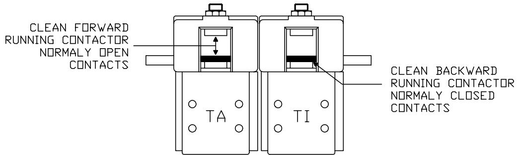
It could be necessary to change both contactors.
