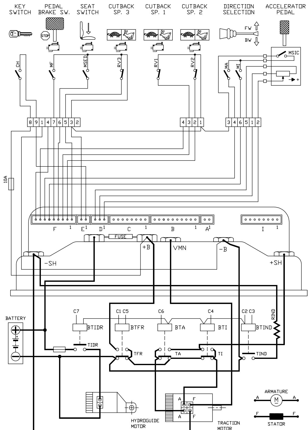
N.B.: The option AUX. FUNCTION must be selected in the HYDRO CONTACTOR mode.
